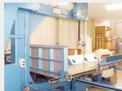
A vertical cutter that can also cut into rounds.
